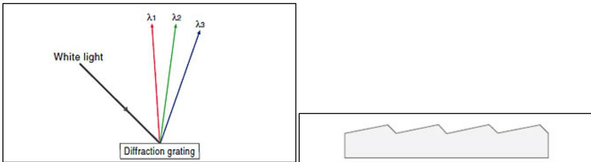
**Figure 2: Scattering of Light Due to Diffractive Pattern & Common Diffractive Pattern Surface<sup>2</sup>**
