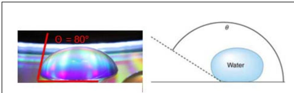
**Figure 4: Contact Angle of Water Drop on CD Surface<sup>3</sup>**
